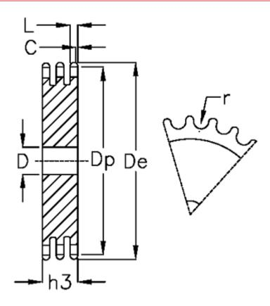
C = 2 D = 30 De = 469.9 Dp = 460.99 For chain size =  $3/4 \times 7/16$ For chain type = 12 B-3 h3 = 49.8 L = 10.8 Number of teeth = 76r = 12.07
